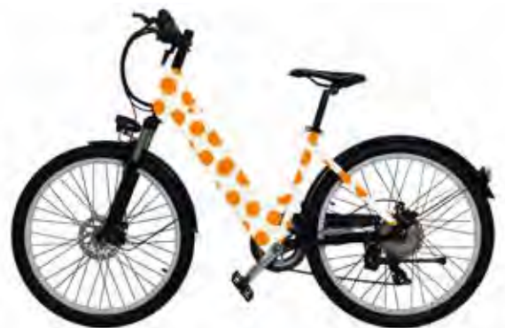
The BSB electric bike has a 30-50km range and a 35km/h top speed.
